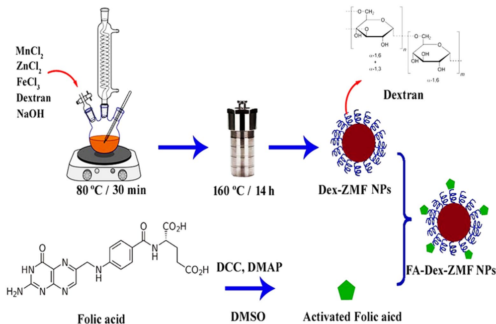
Figure 1. Synthesis process for FA-Dex-ZMF NPs.
